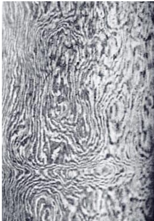
Figure 2: Unique banding patterns on Wootz (source: Wikipedia)
